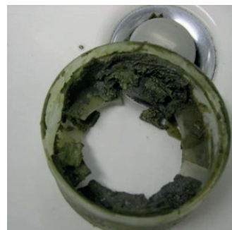
Biofilm on the water deflector of the MST 1
