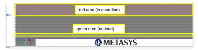
During normal operation (under load) the current should normally not increase above 4A. If the current in no-load operation is above the green area or in the red area (>4A) during normal operation, a service must be done on the module 2.
