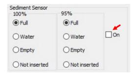
Now the lower light barrier (means 95% full) can then be covered with a screw driver or finger. Now "Full" must be displayed in the area of the 95% light barrier.
