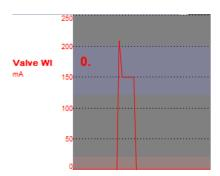
If the valve current is permanent above the blue area (>200mA), the valve must be replaced. Click "On" again to deactivate the valve.
