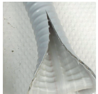
No traces of biofilm in the hose of the suction system
